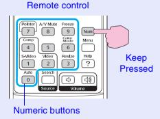
While holding down the [Num] button, press the numeric keypad buttons to enter the password. If the password is entered correctly, projection will start.
