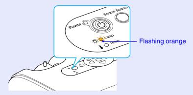
• The projected image gets darker or starts to deteriorate
