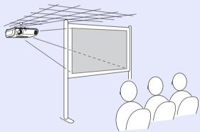
\* A special method of installation is required for suspending the projector from a ceiling. Please contact your supplier if you would like to use this installation method. The optional ceiling mount is required when installing the projector on a ceiling. • p.66
