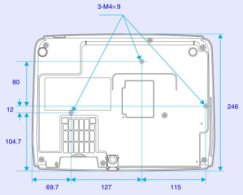
\*Distance from center of lens to suspension bracket fixing point
