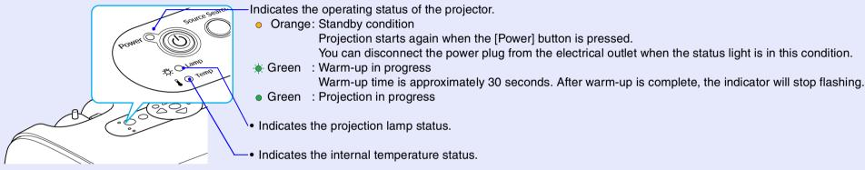
The following tables show what the indicators mean and how to remedy problems that they indicate. If all indicators are switched off, check that the power cable is connected correctly and that power is being supplied normally.
