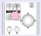
You can reduce the enlarged image by pressing the [-] button. To cancel the E-Zoom, press the [Esc] button.
