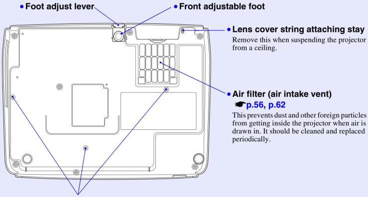
• Suspension bracket fixing points (3 points) p.55, p.66
