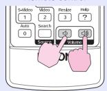
When the button is pressed to the  $[\triangleleft]$  side, the volume increases, and when it is pressed to the  $[\triangleleft]$  side, the volume decreases. The volume gauge appears on the screen when the volume is being adjusted.
